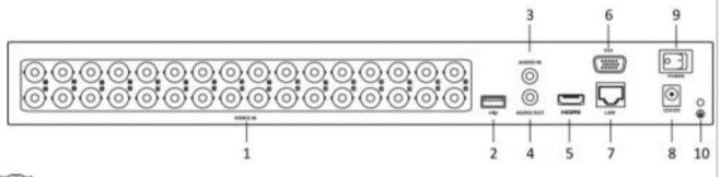
NOTE The rear panel of DVR-224Q-K2 provides 24 video input interfaces.
